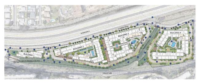
Phase 1 would feature two multi-family residential buildings built on a podium deck over multi-level parking in the central portion of the site and a smaller-scale building in the western-most parcel.
